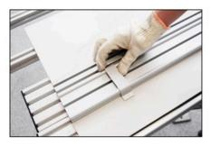
3.Mark the position where you want to cut. Align the edges of the gauge to the position.
