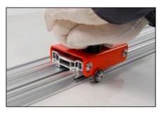
4. Make one continuous motion scoring on the tile with the guide car.
