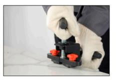
5. Align the center of the separator with the cutting line and apply increasing pressure on it until the tile snaps along the score line. Use pliers to gently clamp the edges of the tile to help it break off.
